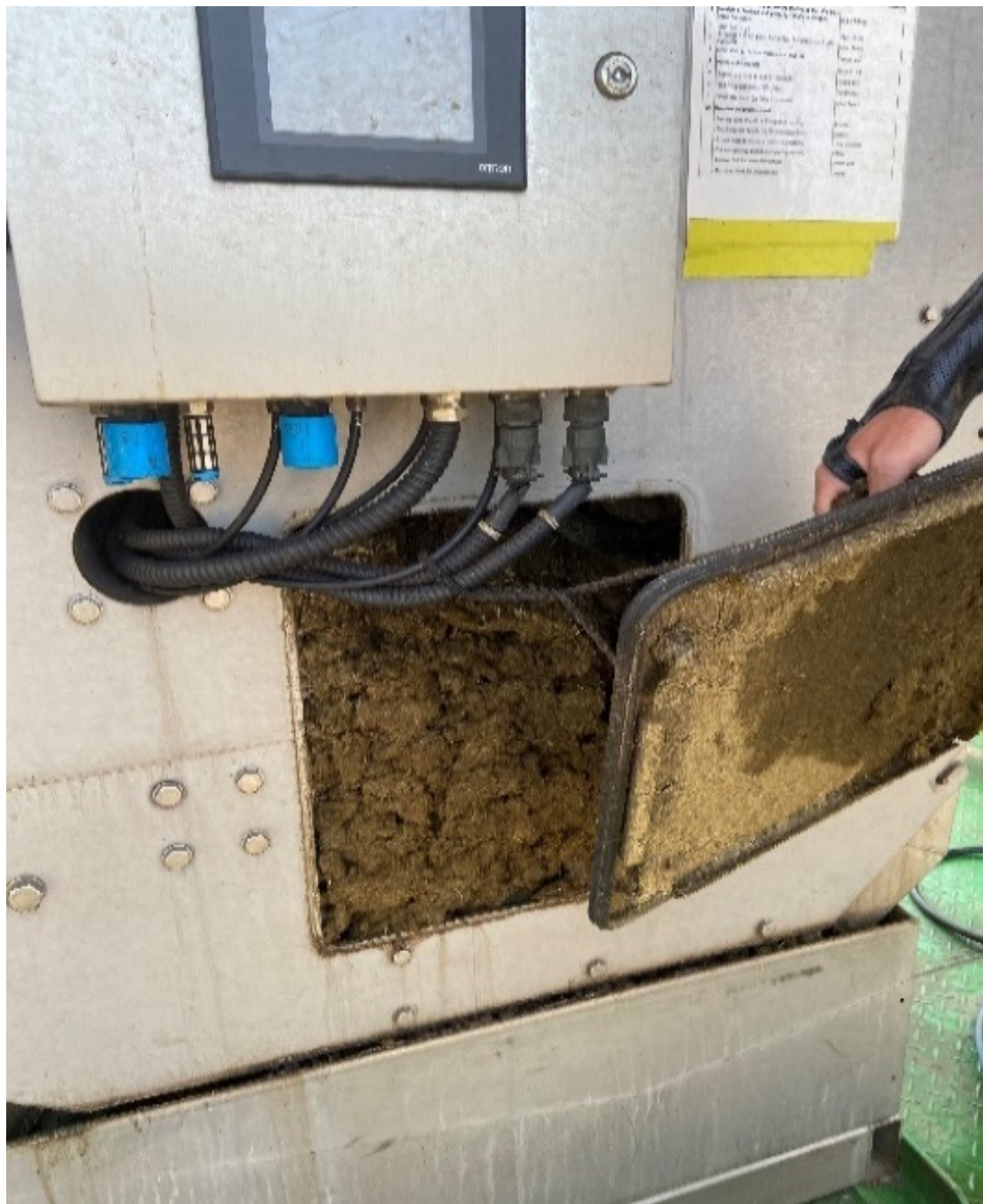
Figure 14 Once during the trial period, the sock became overfilled with manure fibre and dismantled off its runs, opening and emptying manure cake into the Z-Filter internals. This happened unnoticed and led to a substantial amount of manure fibre entering the Filtrate and blocking the onsite irrigation systems.
