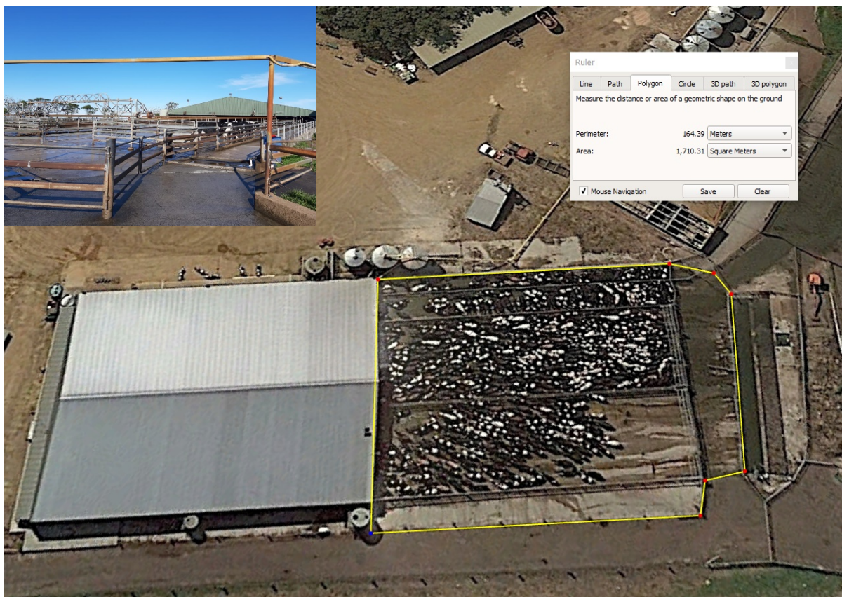
Figure 2 Aerial photo from Google Earth Pro for the milking shed complex showing the estimated catchment area of stormwater entering the effluent management system
