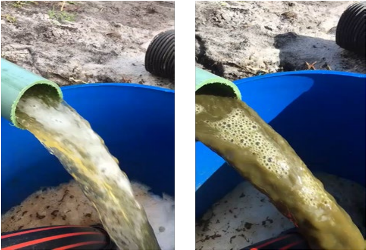
Figure 12 Typical appearance of Z-Filter Filtrate (a) with and (b) without the use of flocculant and lime
