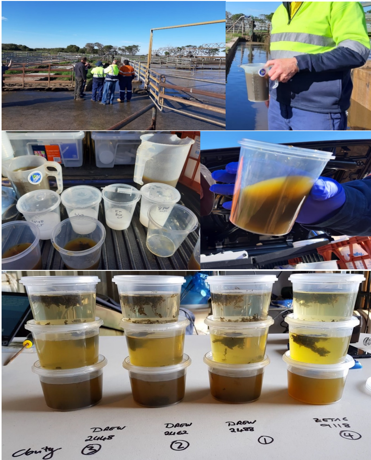
Figure 7 Onsite and offsite testing performed by commercial chemical suppliers SNF and Solenis, to identify suitable chemical recipes to induce separation of manure solids and produce a clear Filtrate
