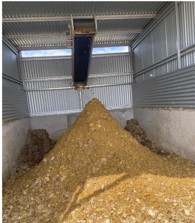
Figure 11 Stockpile of Filter Cake produced by the Z-Filter. The appearance and colour of the Filter Cake is light brown when not using chemicals and dark brown when using chemicals (flocculant+lime).
